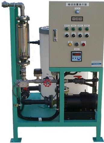
The Anolyte Control System is critical part of the membrane electrode operation. When the process quantity increases, the anolyte conductivity increases. In order to maintain proper operation, the anolyte system must circulate the anolyte at an appropriate rate and discard the anolyte when necessary to keep the conductivity within the desired range.
