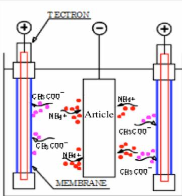
Electrodeposition is a method in which the paint solid is deposited to the articles as the paint solid is drawn by the polarity difference. With this method, an opposite electrode to the article is required. When installed in the ED tank, Tectron® functions as the opposite electrode.
