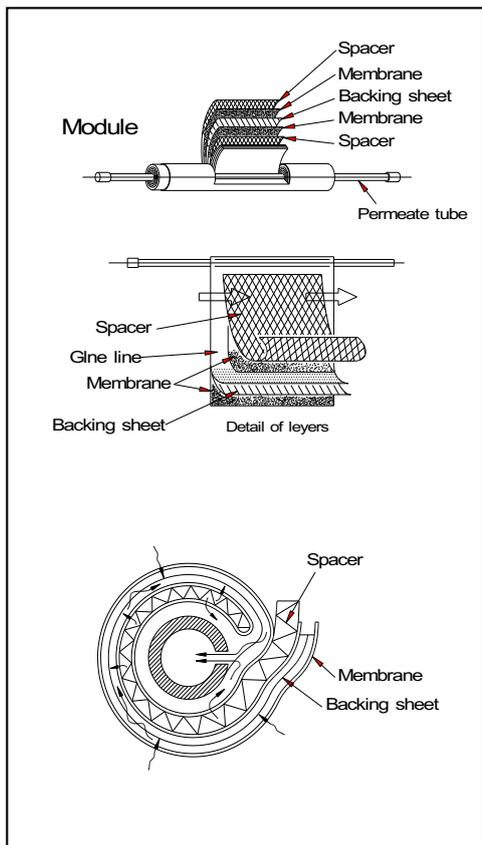
The UF module produces permeate as ED paint flows into the spacer portion of the module and filtered out at the membrane surface.
