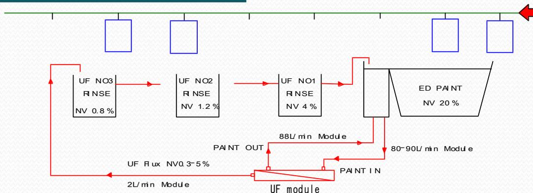
Electrodeposited articles carry out excess ED paint that did not form film. This excess paint is retrieved by rinsing with the UF permeate and returning the rinse solution back to the ED system. This allows the ED system to keep the paint loss at a minimum.
